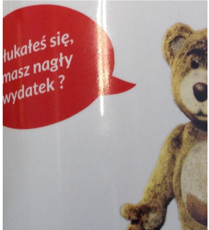
CMYK imprint + additional red ink according to Pantone Matching System (5 colors imprint). Result: clear color as expected.
