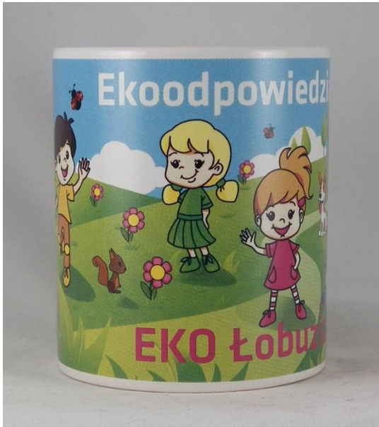
Transfer print (CMYK) – high temperature ceramic decal. Result: Some colors don't meet expectations.
