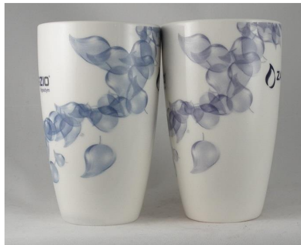
The mugs coming from different production batches (order renewal). Both mugs were made based on the same film.
